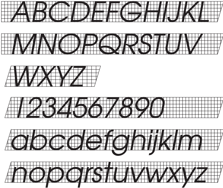
Fig. 34 : Single stroke inclined letters and numerals
