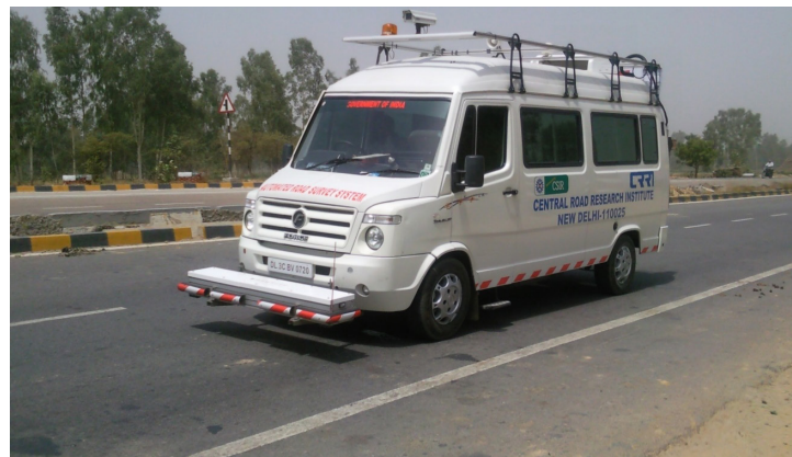
Fig. 1.8. Laser Profilometer Installed in the Front of Survey Vehicle
