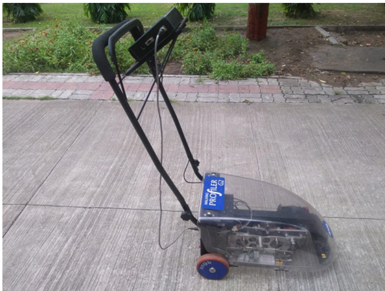
Fig. 1.5. Typical View of Walking Profiler
