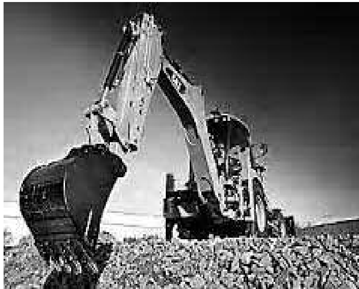
Fig. 1.39. Side shift backhoe hydraulic excavator to dig a straight wall trench on either side of tractor centre.
