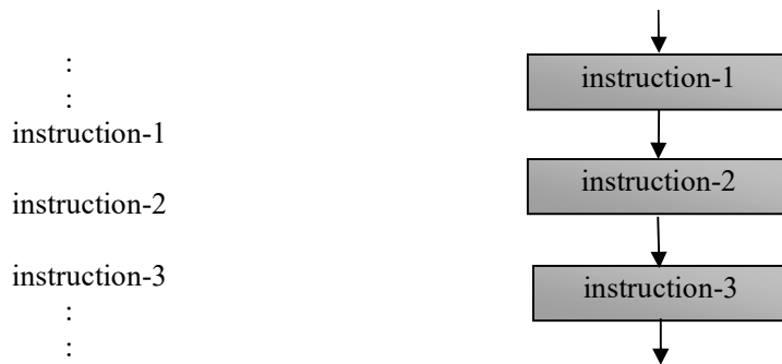
Figure 1.3: Pseudocode and flowchart for sequence structure
