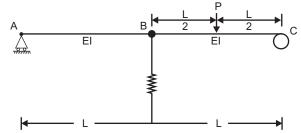
A load P acts at mid point of the rod BC. The downward deflection of joint B is:
