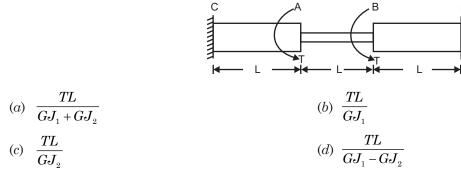
Sol. Part AB simply rotates without any angle of twist. Considering FBD of portion CA,
