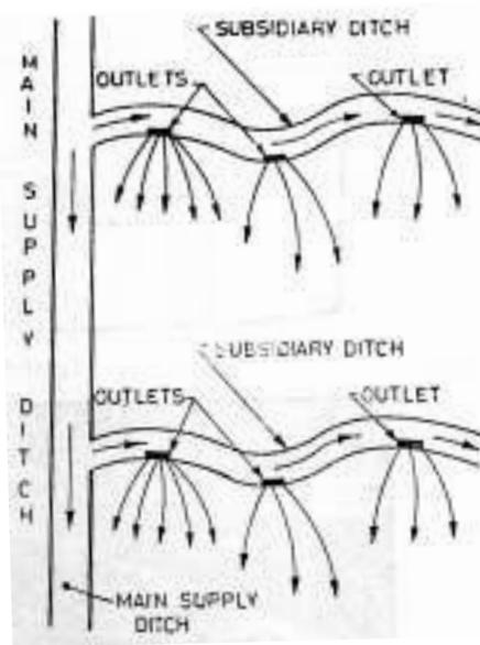
Fig. 1.1. Free flooding (plan view).
