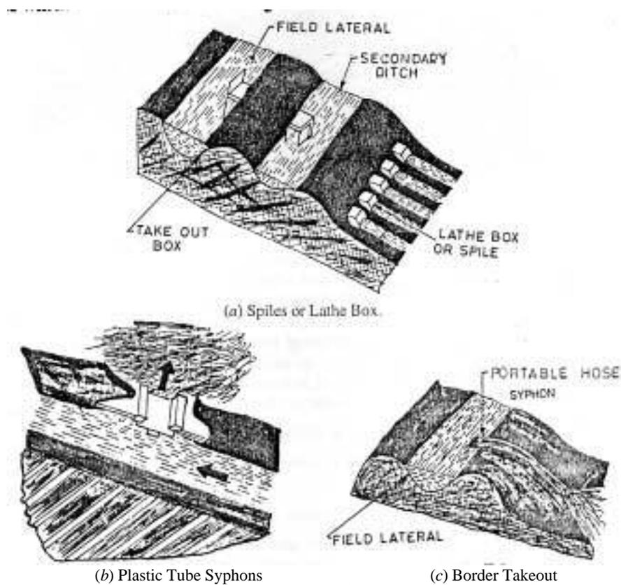
Fig. 1.7. Devices for distributing water from irrigation ditches into fields.
