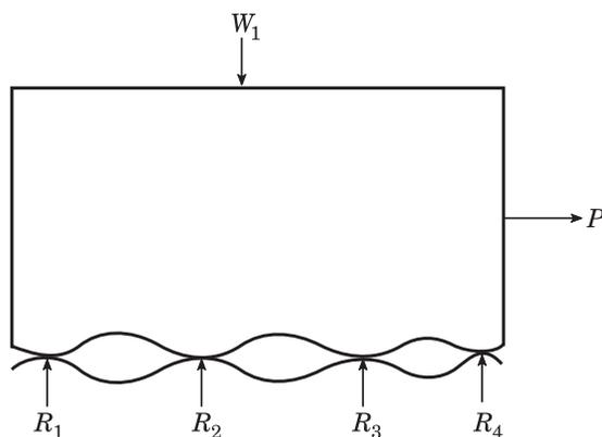
Fig. 1.1. Magnified view of contact surfaces.
