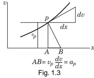
**2. Linear or Angular Motion with Variable Acceleration.** Graphs of above figure indicate relations which apply to linear case.
