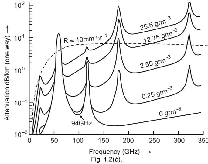
also shows that the excess attenuation above 100 GHz due to rain rate of 10 mm/hr is about 10 dB/km which is around the clear air attenuation with water vapour density of  $25.5 \text{ gm m}^{-3}$ .
