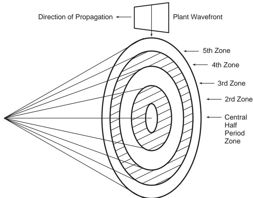
Fig. 1.21. Half period zones for light waves. Light from 3rd zone is cancelled by the 2nd zone, while light from the 5th zone is cancelled by the 4th zone, retaining only the light from the 1st half period zone, which propagates, in a straight line path along the direction of propagation.
