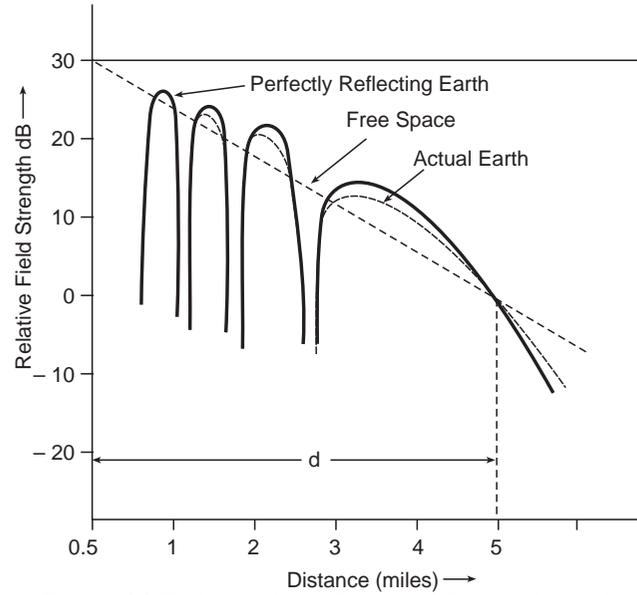
Fig. 1.26(a) Field strength as a function of distance, flat earth.
