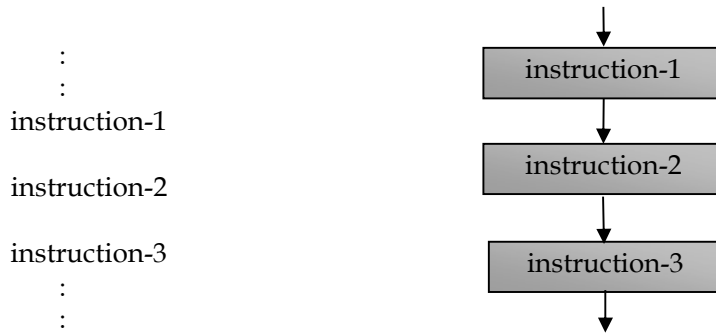
Figure 1.3: Pseudocode and flowchart for sequence structure
